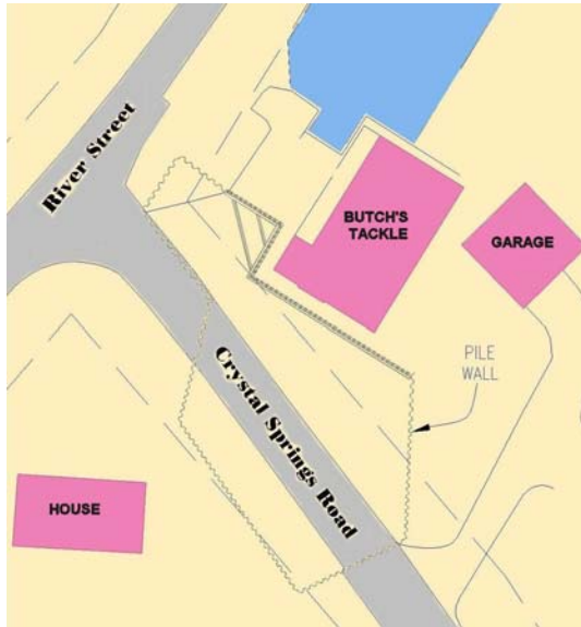
Site sketch showing proximity of the proposed pile walls to the buildings
